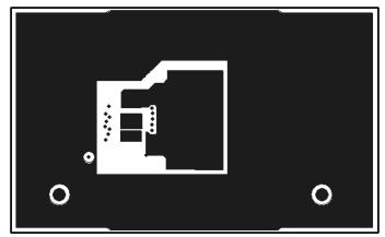
Figure 18. SP7663EB PC Layout 3rd Layer Side
