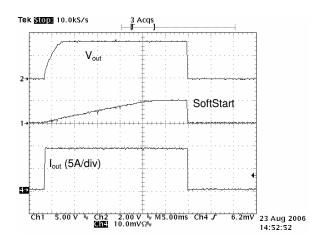
Figure 5. Current Limit set point 9A
