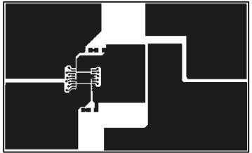
Figure 16. SP7663EB PC Layout Top Side
