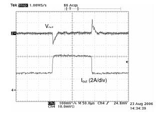
Figure 3. Load Step Response: 3->6A
