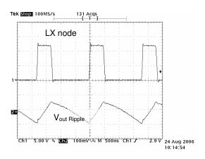
FIGURE 12 VOUT RIPPLE LX NODE 0A OUT
