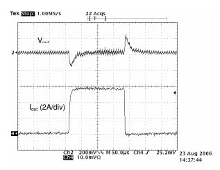
Figure 4. Load Step Response 0->6A
