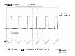
Figure 2. LX node output ripple voltage
