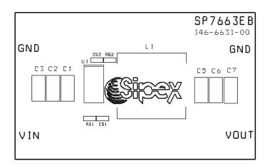
Figure 15. SP7663EB Top Side Component Placement
