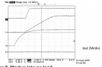
Figure 8. Startup into no load
